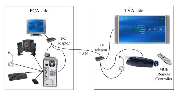
There are two adaptors, PC adaptor and TV adaptor, and two displays, a monitor and a TV, are connected to each adaptor. The PCA will process EDID and let the PC know what kind of resolutions can be supported. The rules are describes below.
